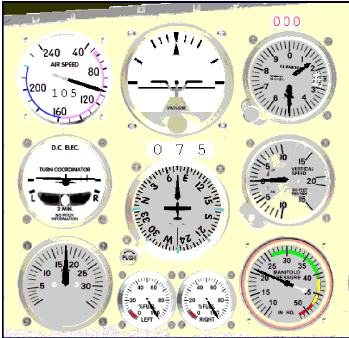
Slow-flight: 1800 RPM, 21 in. M.P., 105 kts.
