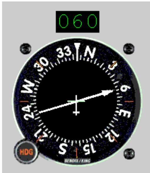
RMI, Radio Magnetic Indicator
