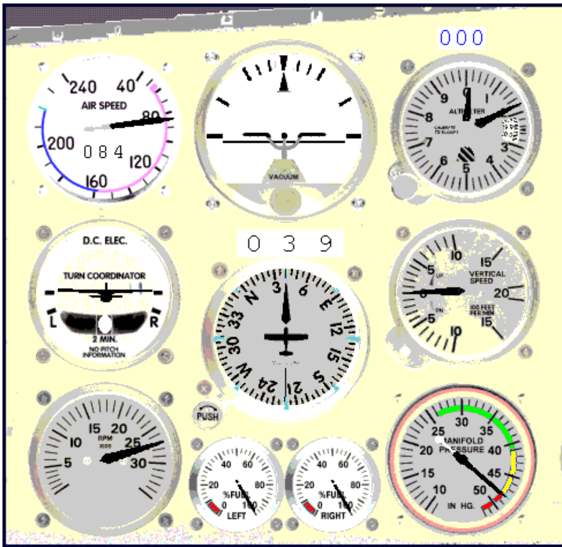
Takeoff: 2700 RPM, 48 in. M.P. Lift off at 84 knots.
